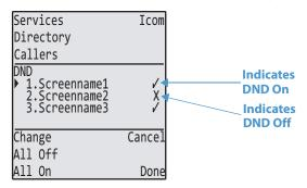
In the above example, Screenname 1 and 3 have DND ON as indicated by a check mark ( $\checkmark$ ). Screenname 2 has DND off as indicated by an **X**. The ALL ON and ALL OFF softkeys allow you to enable or disable DND on all accounts, respectively.
