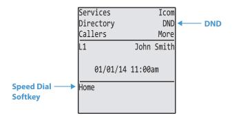
You can configure up to 10 functions on the top set of softkeys. If you have additional functions configured on the top softkeys that do not display on the main idle screen, a "**More**" displays at the top right of the screen. Pressing the **More** softkey toggles between the first screen and a second screen of softkeys configured on your phone.
