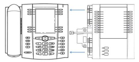
The M675i provides 10 softkeys in each column (totalling 20 keys) on the keypad. The M675i also provides 3 keys at the bottom left of the unit. These keys represent "Page 1", "Page 2", and "Page 3" of the LCD display. The M675i has 20 keys available on each page (totalling 60 softkeys). Each key provides an LED for indicating call status. The M675i provides an LCD for displaying key labels.
