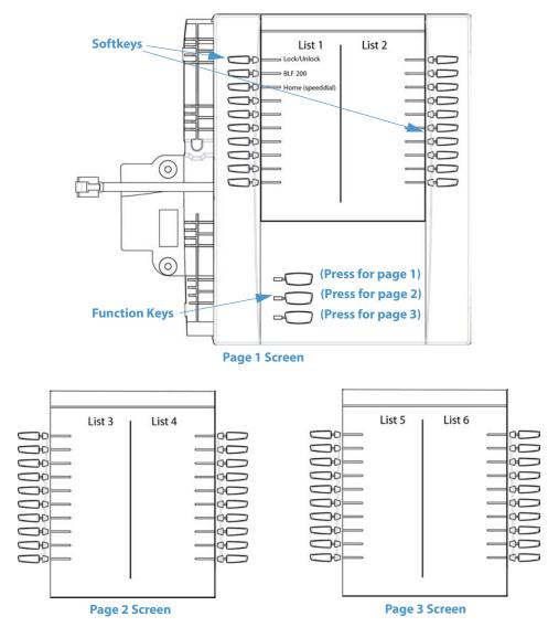
To use the M675i, press the function key for the page you want to display to the LCD (page 1, page 2, or page 3), and press the applicable softkey.
