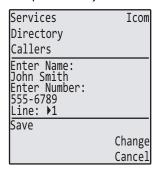
This is the line that the phone opens to dial the number after you press the speed dial key. By default, the phone uses Line 1 for the speed dial key. If you want to use a different line, press the "**Change**" key, or press the ▶key to select another line.
