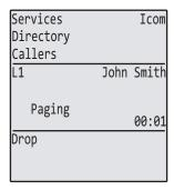
2. Press the **Drop** key to end the multicast RTP session and return to the idle screen.
