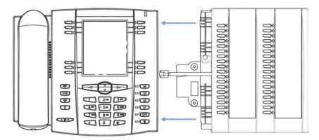
The M670i provides 18 softkeys in each column (totalling 36 keys) on the keypad. Each key provides an LED for indicating call status. The M670i provides a paper label for convenient key labelling.
