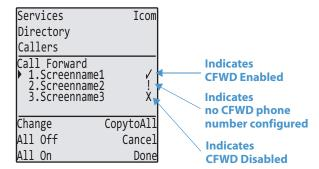
In the above example, Screenname 1 has one or more CFWD states enabled as indicated by a check mark ( ), Screenname 2 has one or more CFWD states enabled but a specific state has no call forward phone number configured as indicated by a , and Screenname 3 has one or more CFWD states disabled as indicated by an **X**.
