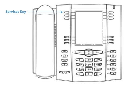
Using the Aastra Web UI, you can configure a key to access XML applications. Under *Operations->Softkeys and XML* or *Operations->Expansion Module*, you can assign a key the type "XML".
