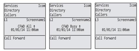
In the above example, Screenname1, Screenname2, and Screenname3, are three accounts configured on the phone. Screenname1 has "CFWD All" enabled, Screenname2 has "CFWD Busy" enabled, and Screenname3 has CFWD disabled as indicated by no message displayed.
