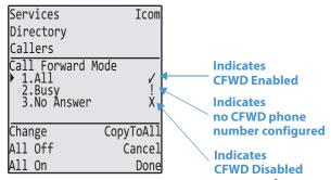
In the above example, **CFWD All** is enabled as indicated by a check mark ( $\checkmark$ ), **CFWD Busy** is enabled but no call forward phone number is configured as indicated by a  $\frac{1}{2}$ , and CFWD No Answer is disabled, as indicated by an  $\frac{1}{2}$ .
