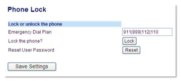
2. In the "Emergency Dial Plan" field, enter the 3-digit number used in your local area to contact emergency services. For multiple numbers, enter a "|" between each emergency number. For example: 911|110
