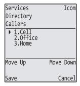
• Pressing the **Save** softkey in the above screen places the Cell label, the Cell number, and line associated with the Cell number, into the one position. So the first screen to display for the entry would be the Cell number screen. If no label is assigned to the entry, the numbers would be arranged in the order you specify.
